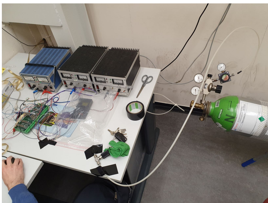
Figure 5.15: Setup used for the test of the humidity sensors. On the desk you can see the ELMB, which was used to readout the HM1500LF and the HIH-4000 humidity sensors. The three sensors were placed inside the plastic bag and the gas was inject with the help of the bottle on the right.
