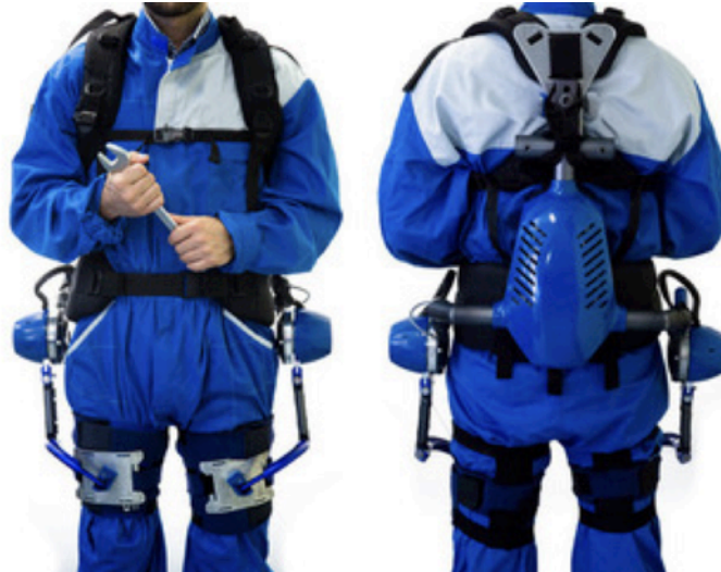
Figure 6.4 The Robo-mate mk2b prototype is an intermediate version of the evolution from the Robo-Mate prototype to XoTrunk, as presented in Chapter 3.
