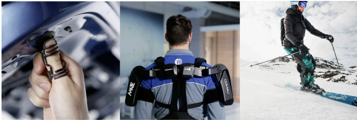
Figure 2.2 (left) Ottobock Paexo Thumb, the smallest exoskeleton in the world for transferring forces from the thumb to the entire hand. Image credit: Ottobock; (middle) Comau Mate, a shoulder exoskeleton for assisting the worker in overhead tasks. Image credit: Comau; (right) Roam Elevate, the exoskeleton supporting skiers' knees and quads during downhill skiing. Image credit: Roam robotics
