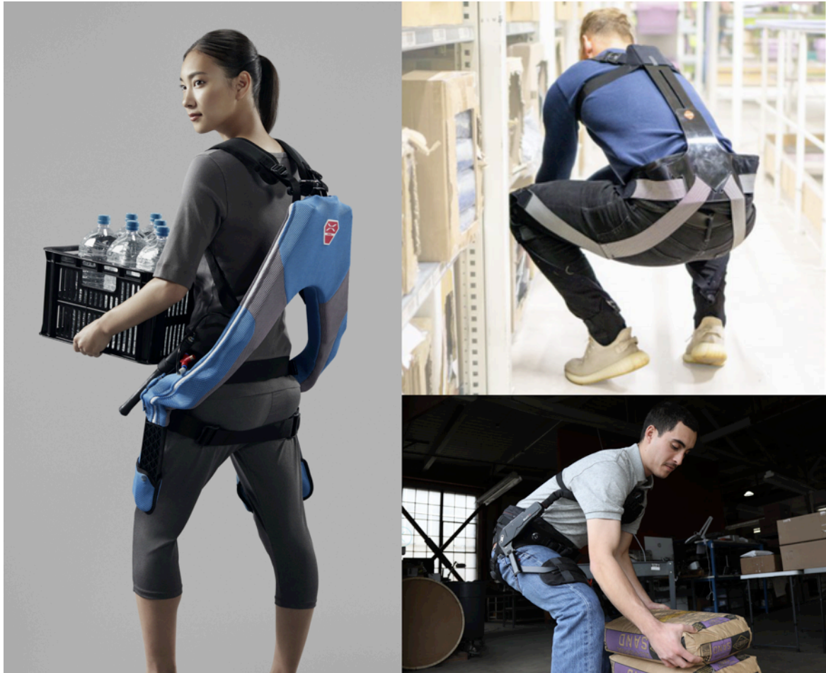
Figure 2.5 (Left) Innophys Muscle Suit Every. Image credit: Innophys. (Right, top) Hunic SoftExo. Image credit: Hunic. (Right, bottom) SuitX backX. Image credit: SuitX.
