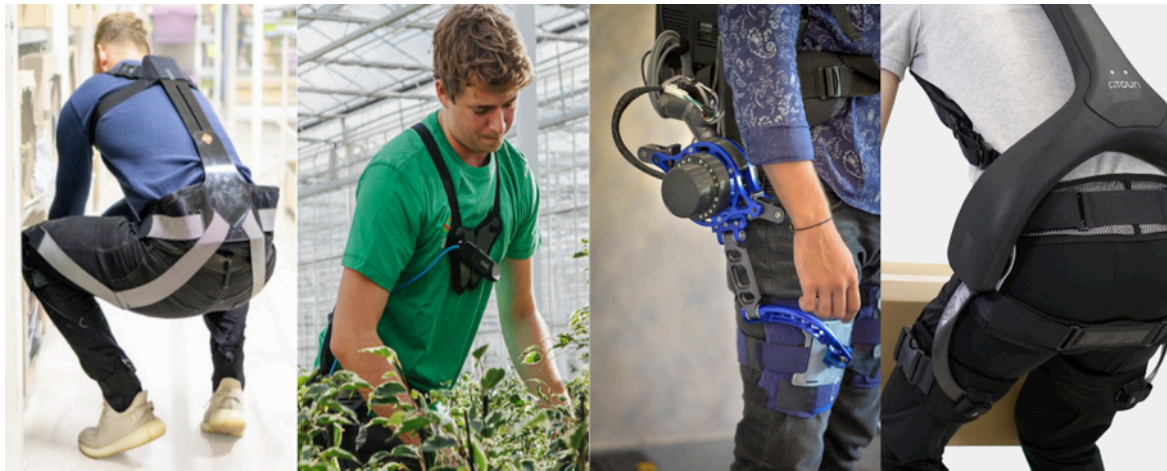
Figure 2.4 Representation of a soft and three rigid exoskeletons and some implementation details. From left to right: (i) Hunic SoftExo (image credit: Hunic), an example of soft exoskeleton where the trunk extension is supported pulling from the shoulders; (ii) Laevo v2.5 (image credit: Laevo), an example of rigid exoskeleton where the trunk extension is supported by pushing on the chest; (iii) Robo-Mate Trunk module (image credit: robomate.eu), an example of rigid exoskeleton that assists hip extension by pushing on the thighs; (iv) Atoun Model Y (image credit: Atoun), an example of rigid exoskeleton that supports hip extension by pulling from the thighs. Also note how Robo-Mate and Atoun present a lumbar cushion and a buttocks belt, respectively.
