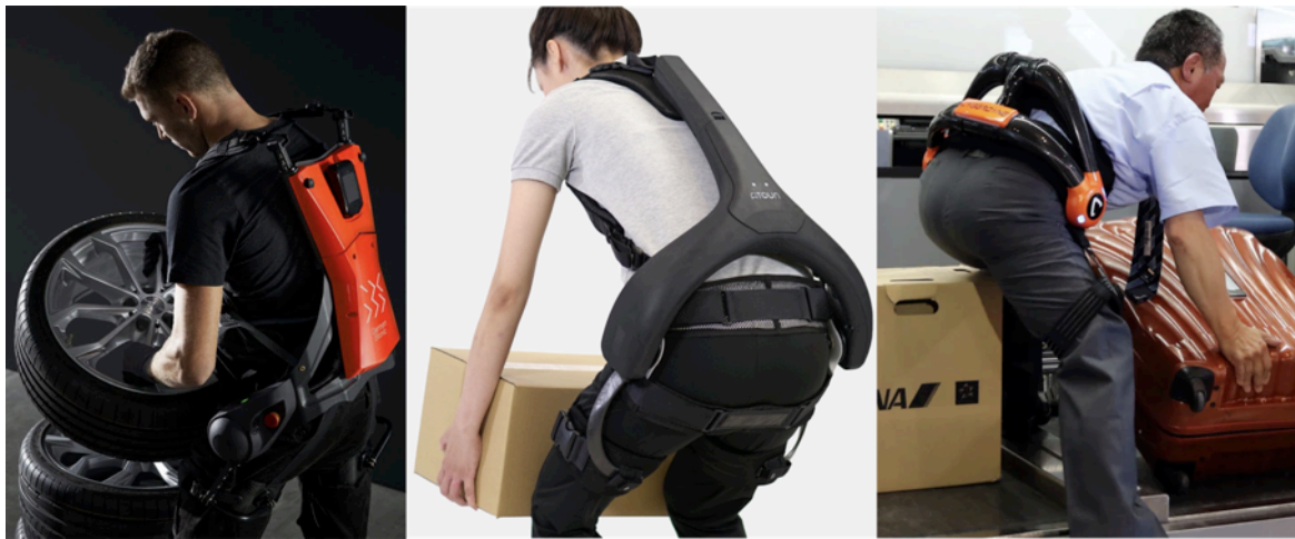
Figure 2.6 (Left) GBS Cray X. Image credit: GBS. (Centre) Atoun Model Y. Image credit: Atoun. (Right) Cyberdyne HAL for labour support. Image credit:aviationpros.com
