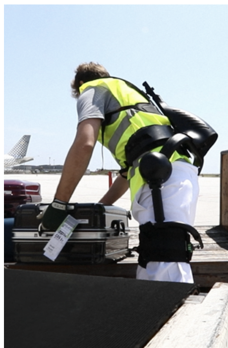
(a) Robo-Mate usage during warehouse pick and place (b) XoTrunk usage during the loading of an aircraft hold.
