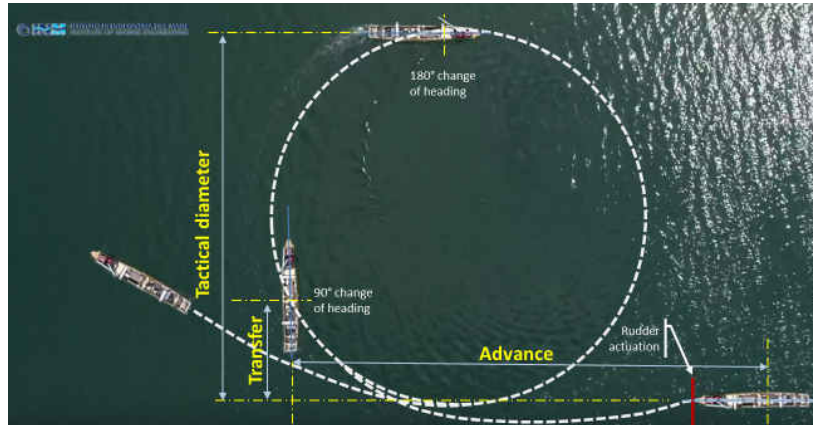
Figure 3.2 Turning circle main quantities
