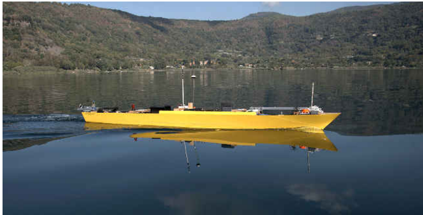
(a) Scaled model during free running tests
