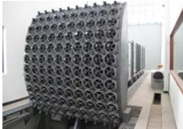
FIGURE 6.8: Wall of fans of the Multiple-fan wind tunnel of Tongji University, (S. Cao and J. Cao, 2017).
