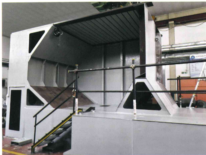
Figura 4 - Fotografia del modulo principale della testing facility (dimensioni principali LxWxH 7000x4000x4000 mm). Figure 4 - Photo of the main module of the testing facility (main dimensions LxWxH 7000x4000x4000 mm).
