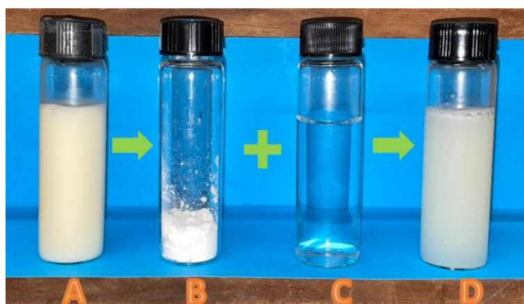
Figure 58. From emulsion to powder and back to emulsion steps. A) loaded nanoemulsion with 40 % (w/w) of maltodextrin, B) dried powder, C) water, D) nanoemulsion rehydration.
