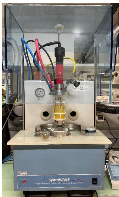
Figure 8. MW multimodal reactor: SynthWAVE, Milestone, Bergamo, Italy.
