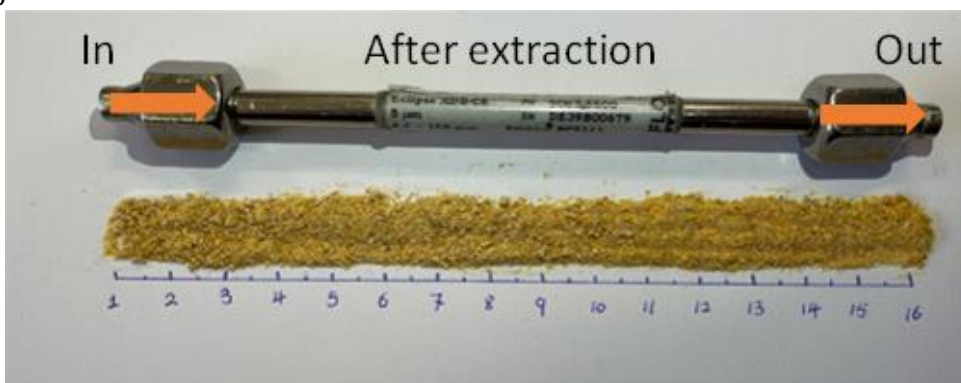
Figure 30. Tomato waste. a) without extraction, b) after 3 hours extraction with ethanol.
