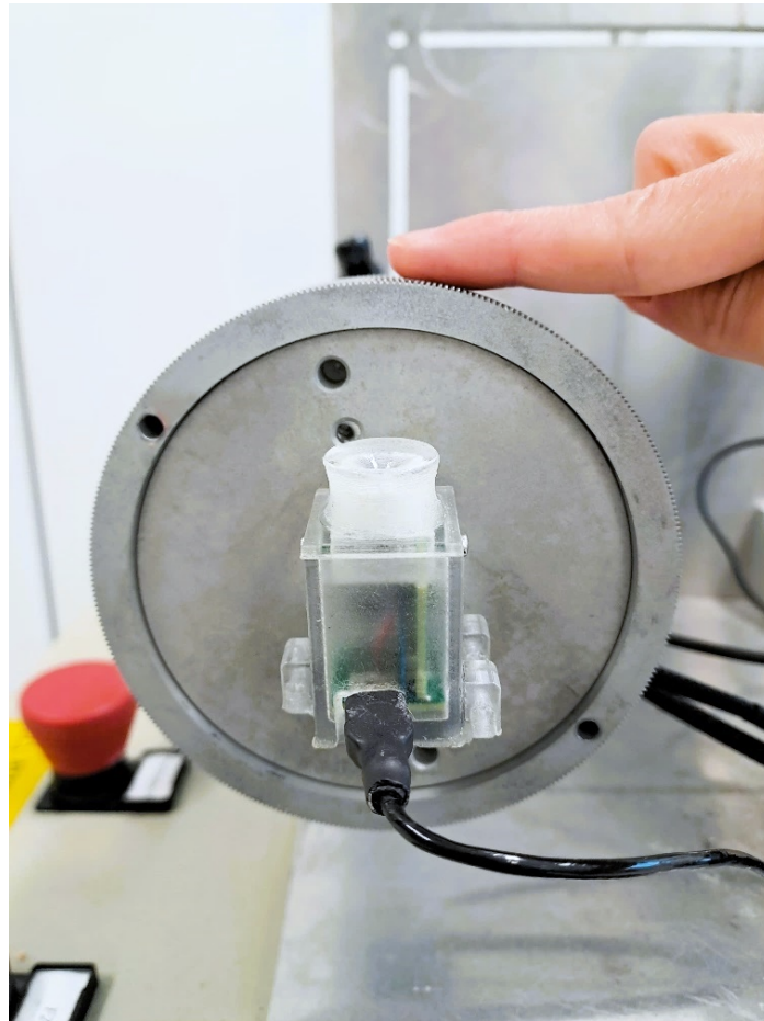
Figure 2.4 Experimental setup consisting a wheel with a gearing of 10 cycles/cm and a module of MSI Caterpillar.
