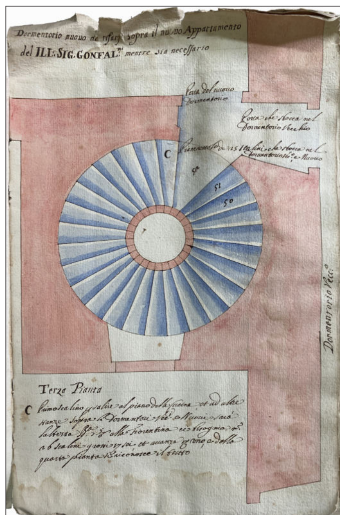
Figure 18: Plan of the third level of the spiral staircase built at the back of Pistoia’s communal palace, 1681 (Raccolte 4: 147r). Courtesy of Ministero della cultura, Archivio di Stato di Pistoia, prot. n. 1329–2024.
