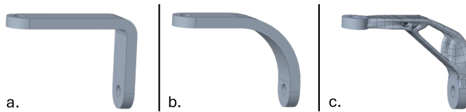
Fig. 6. a) Original Inversion Lever, b) Inversion Lever optimized traditionally, c) Inversion Lever GD optimized.
