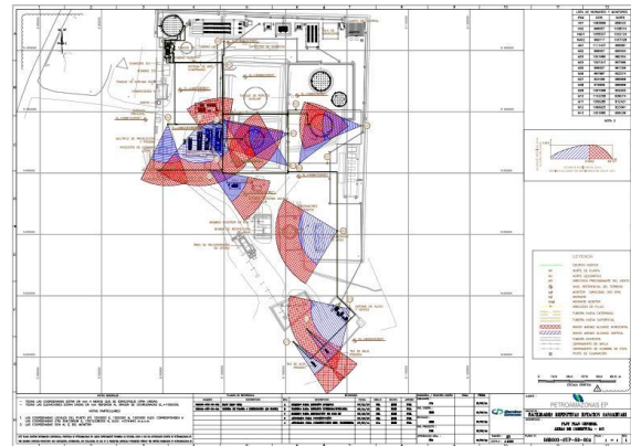
Figure 4. Plant Fire System Coverage
