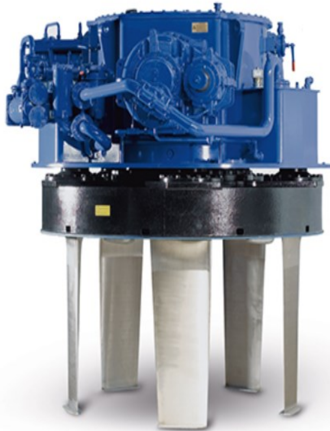
Figure 1.2: Cycloidal propeller (Intelligent Propulsion System for Safe Shipping, Voith Turbo Schneider Propulsion, brochure).
