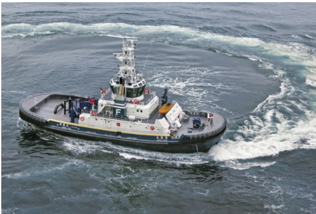
Figure 1.7: Water tractor equipped with epicycloidal propellers ( http://www.voith.com )
