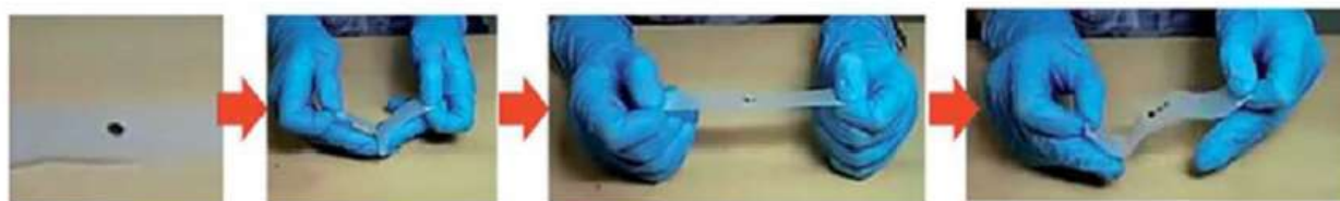
Figure 1.5 Photographs of illustrative procedure of mechanical exfoliation. 127
