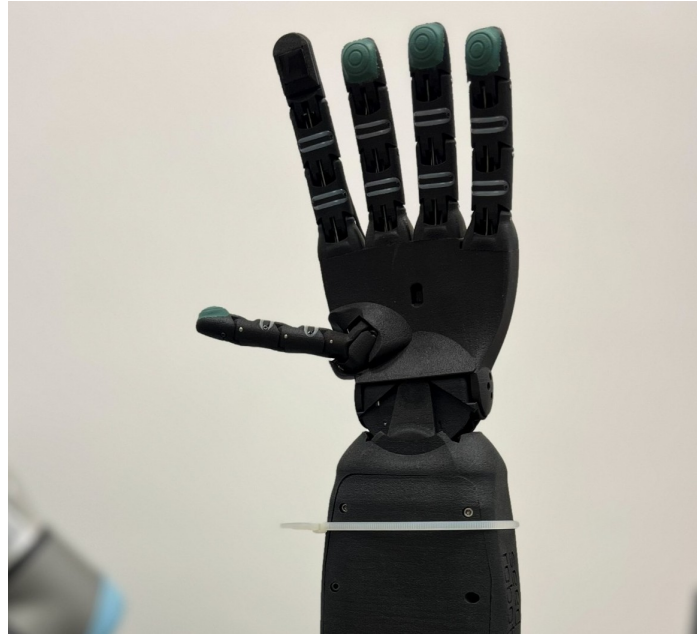
Figure 5.5 Integration of compact fingertip on index finger of SEEDs anthropomorphic Hand
