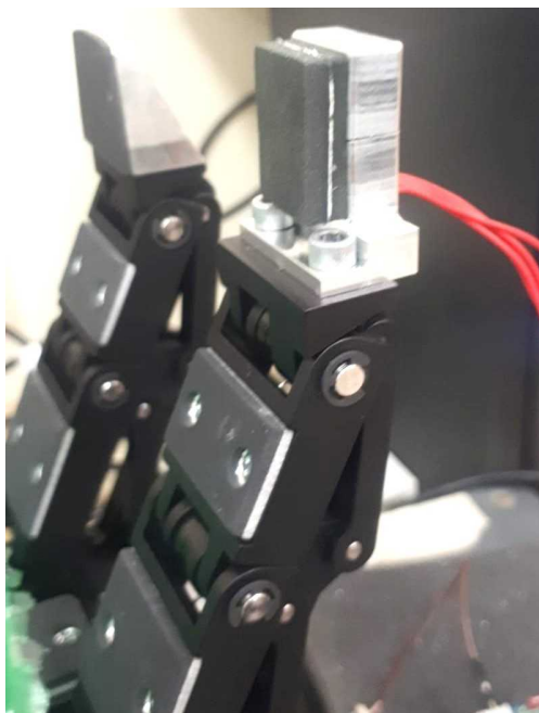
Figure 3.6 Mechanical integration within three-fingers adaptive gripper
