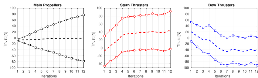
Figure 11. Convergence of the forces of each actuator (circle for rithy and square for the left side).
