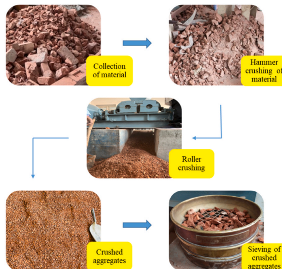
Fig. 1. Production process of RBA
