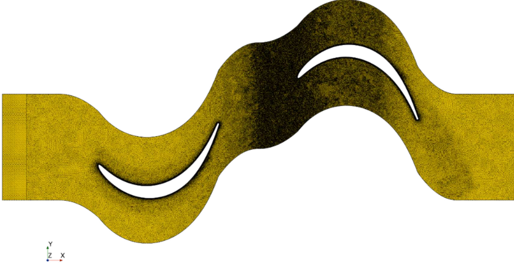
Figure 6.1: Schematic of an exemplary stage-like simulation environment for unsteady inflow conditions
