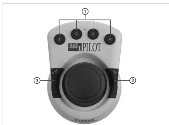
Figure 2. Picture of the IMAGE1 PILOT. 1) Programmable buttons (1-4) for quick access; 2) ESC button; 3) ENTER button.
