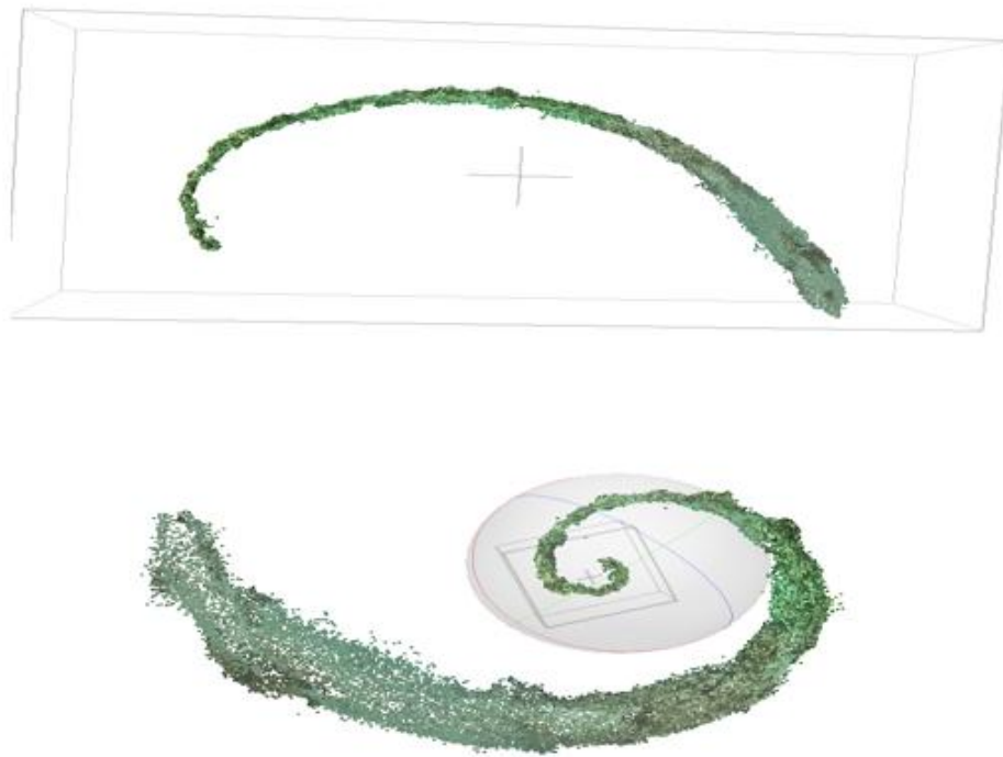
Figure 36. Image from Agisoft Metashape© (V 1.8.2) showing the tie points obtained with automatically computed camera calibration parameters (side view for both panels).
