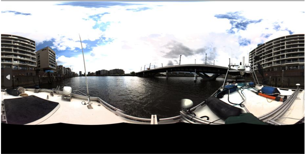
Figure 49. Panoramic image from the 360° camera taken from the boat. The boat appears in white and must be masked for proper photogrammetric processing.
