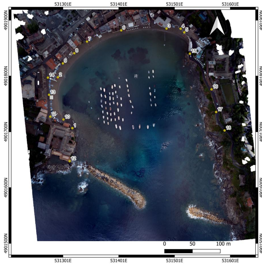
Figure 14. Orthophoto with the distribution of GCPs (yellow dots with numbers along the coast) in the study. Water refraction not taken into account.
