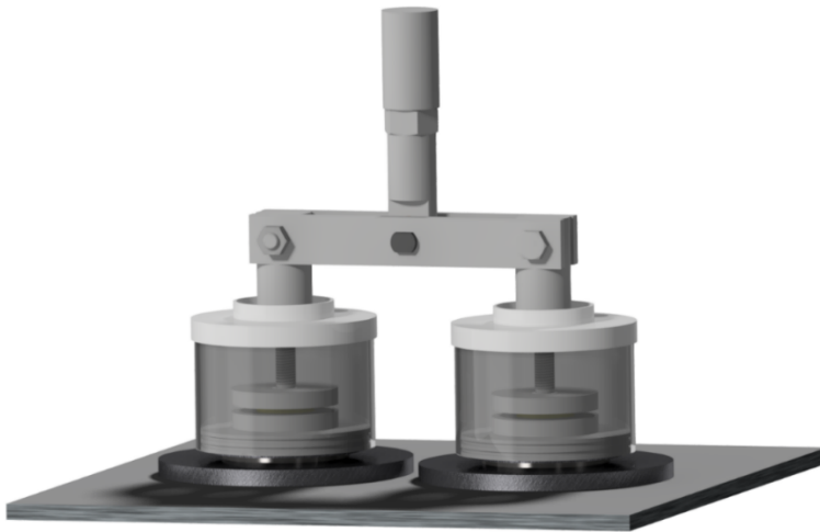
Figure 4.2: Developed test setup to simultaneously induce a compression and a stretching in two fatigue-ring specimens.
