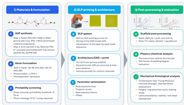
Figure 4.1: Schematic overview of the digital light processing (DLP) workflow for the fabrication and evaluation of acrylate-terminated urethane-PEG (AUP) scaffolds. The process includes (1) AUP synthesis and resin formulation, (2) DLP printing and architectural design, and (3) post-processing and physico-chemical, mechanical, and biological characterization.
