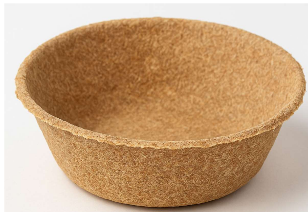
Figure 13. Biodegradable recipient made from the F1 biocomposite (80% cassava residue—CR, 5% bacterial cellulose—BC, and 15% sugarcane bagasse—SCB).
