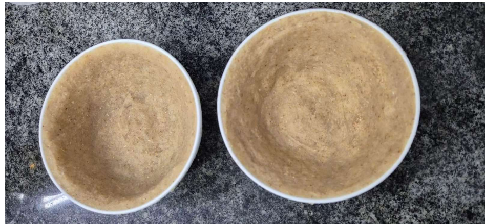
Figure 12. Molding step of biocomposite.
