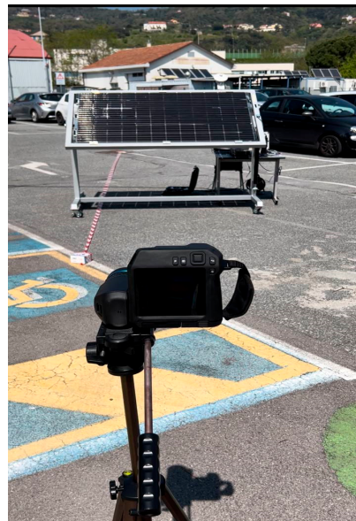
Figure 8. Experimental setup at the University of Genova Savona Campus showing the bifacial PV mobile bench oriented at an azimuth angle of +60° facing southwest, with the FLIR thermal camera mounted on a tripod at 6 m.
