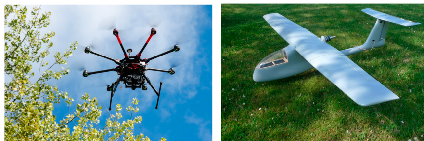
Figure 21. UAV types used in PV inspection: (left) multirotor hexacopter ideal for detailed, localized monitoring; (right) fixed wing UAV suitable for long range, large area surveillance [112].
