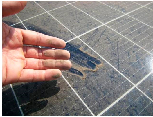
Figure 16. Accumulated dust on different PV modules installed in Kuwait, showing varying soiling patterns and intensities.
