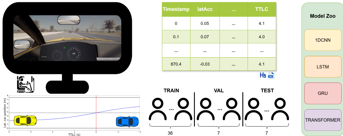
Fig. 4.1 Pipeline of driving simulation, data collection, and model training.
