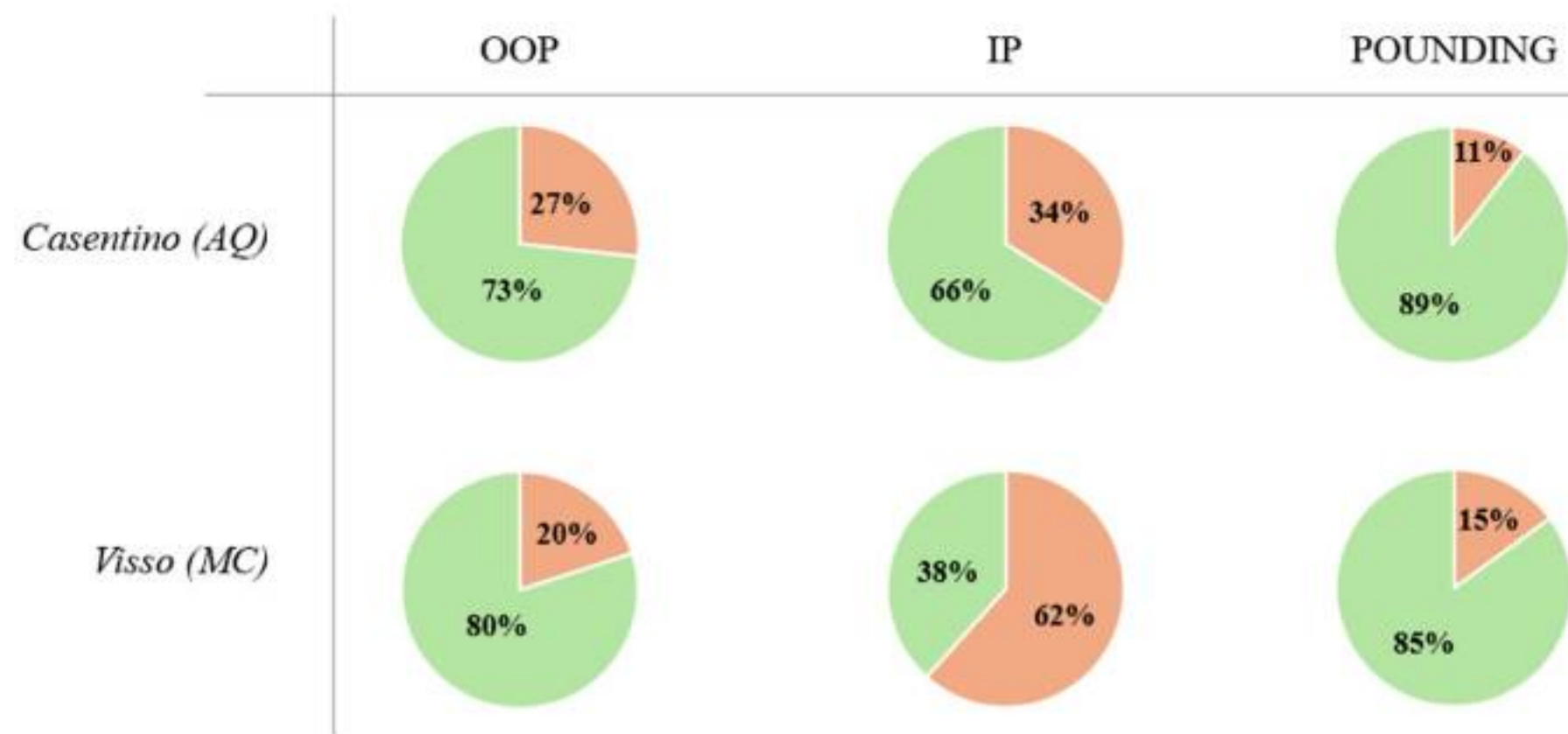
Fig. 13. Graphical representation of damage activations for IP, OOP and pounding in the historic centers of Visso and Casentino.
