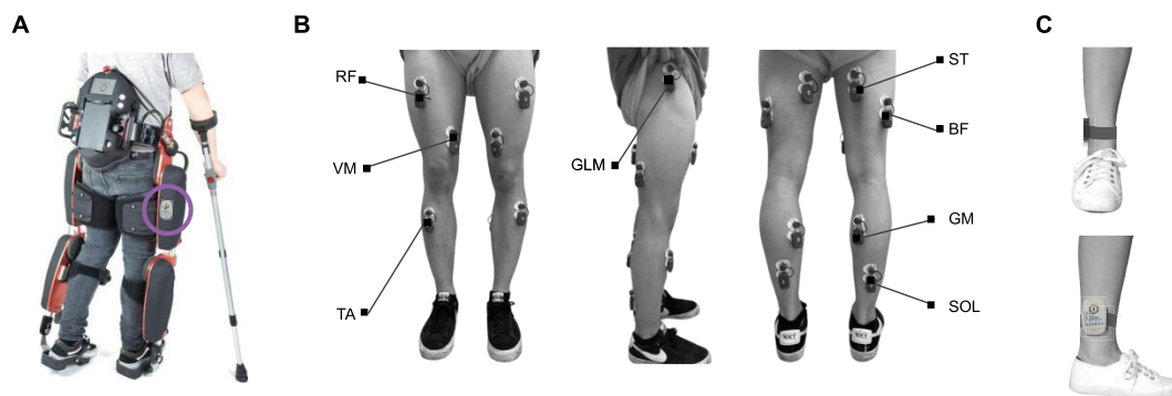
FIGURE 1. Experimental setup. Panel A: UAN.GO exoskeleton and Inertial Measurement Unit (IMU) placement (purple circle) during exoskeleton walking. Panel B: Placement of surface electromyographic (EMG) electrodes, recording bilaterally from tibialis anterior (TA), gastrocnemius medialis (GM), soleus (SOL), rectus femoris (RF), vastus medialis (VM), semitendinosus (ST), biceps femoris (BF), and gluteus medialis (GLM). Panel C: IMU placement during normal walking, frontal (top panel) and lateral view (bottom panel).
