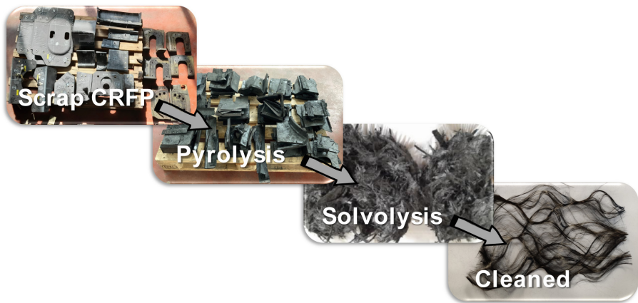
Fig. 2. Process diagram of the carbon fibre recycling process.
