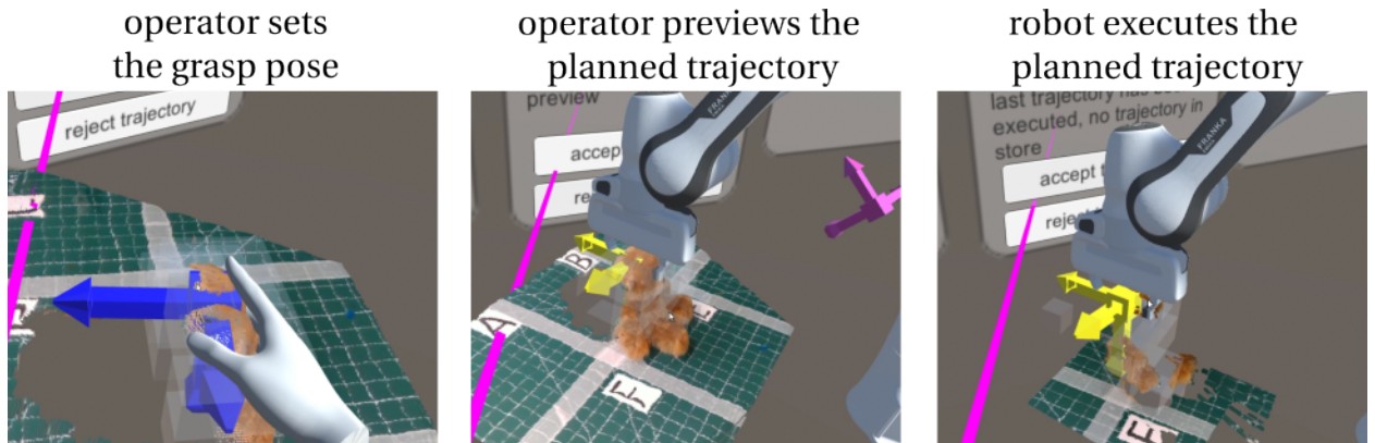
Figure 2.8: Supervised control mode: move-to-grasp.
