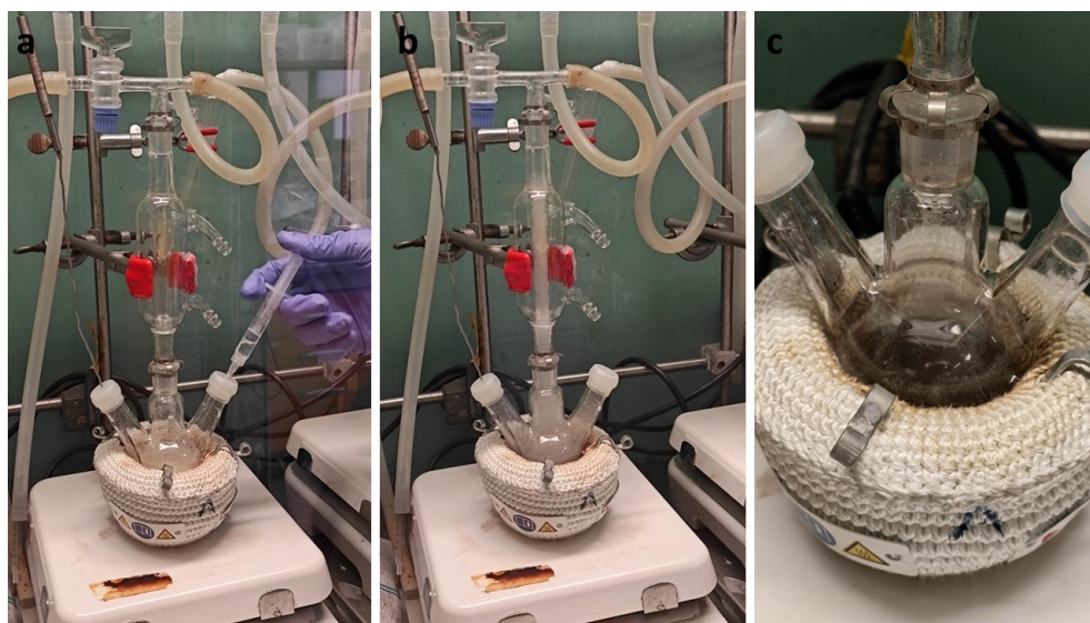
Figure 3.3.9. Images of the reaction setup (a) before injection, (b) immediately after injection, and (c) 5 minutes after the injection of 0.8 mmol of TOA- \text{AlH}_3 into the reaction mixture. In contrast to the behavior observed with DMEA- \text{AlH}_3 , the images demonstrate stable reaction conditions with no boiling bursts or disturbance of the reaction setup.
