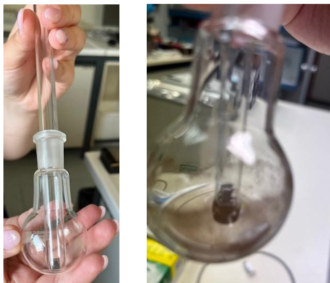
Figure S10: Recovery system to separate biocatalyst from reaction
