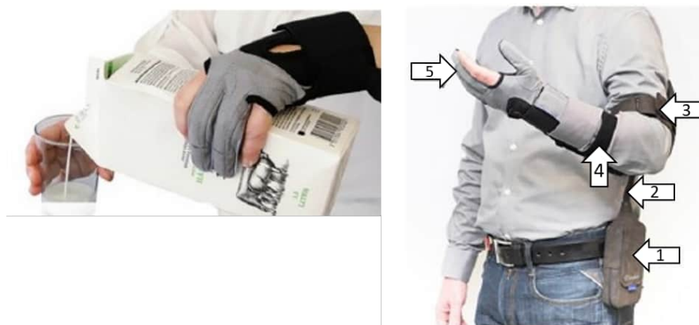
Figure 27. The Bioservo Carbonhand ® device and examples of related applications [54]. Legend: (1) SEM unit; (2) cord; (3) arm strap; (4) slap wrap; (5) glove, three-finger version.
