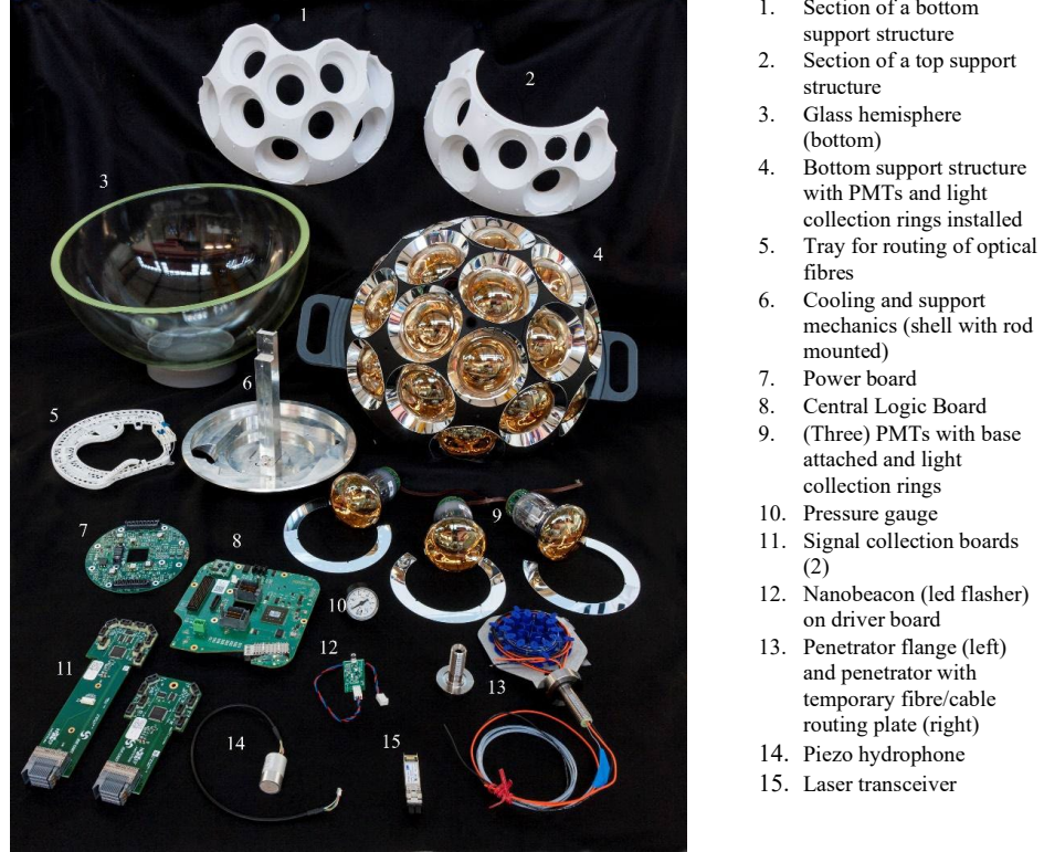
Figure 2.14: Photo of a selection of components of an optical module [182].
