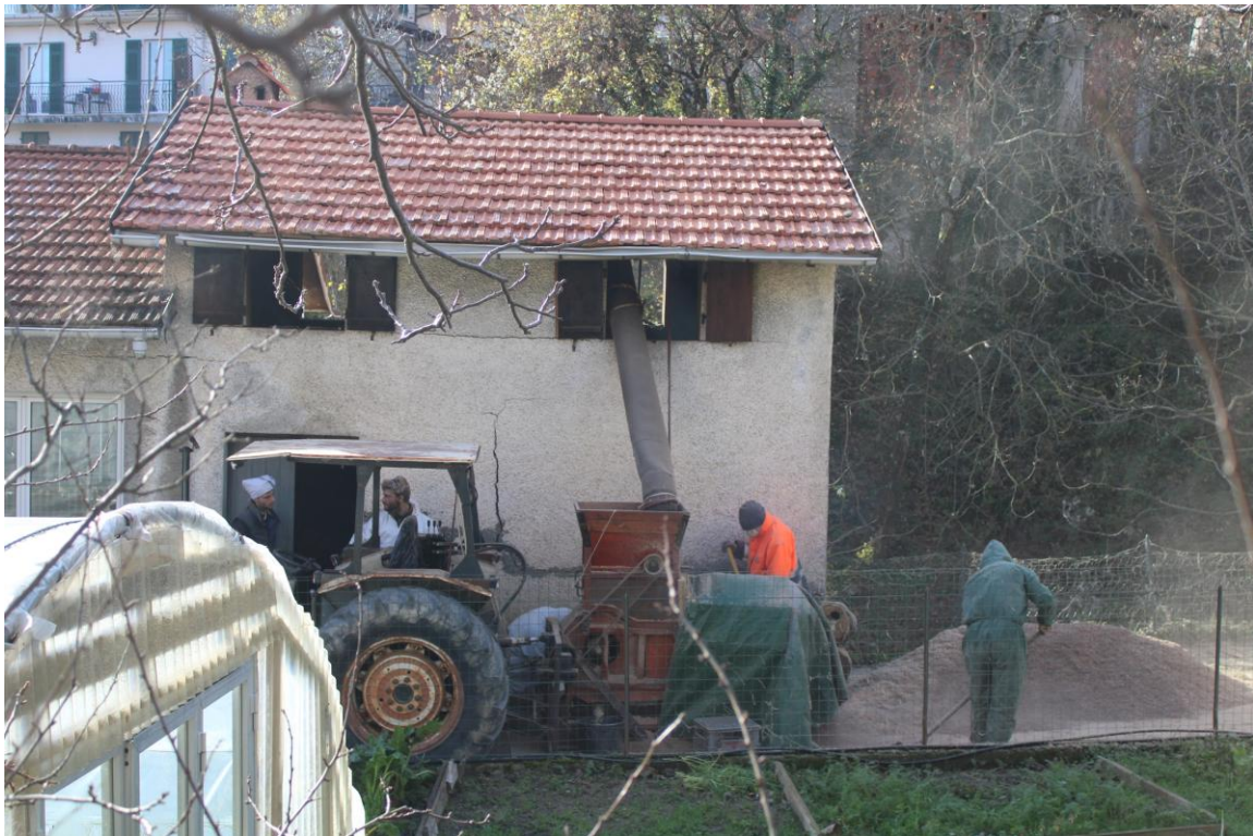
Fig. 4.3.12. Chestnuts beating in Campore (Maissana). The beating machine is connected directly to the dryer through the window, from which the chestnuts, still warm, are fed in to be beaten. On the right, the waste and dust expelled by the machine are piled up. Source: Author's photograph, December 2025.
