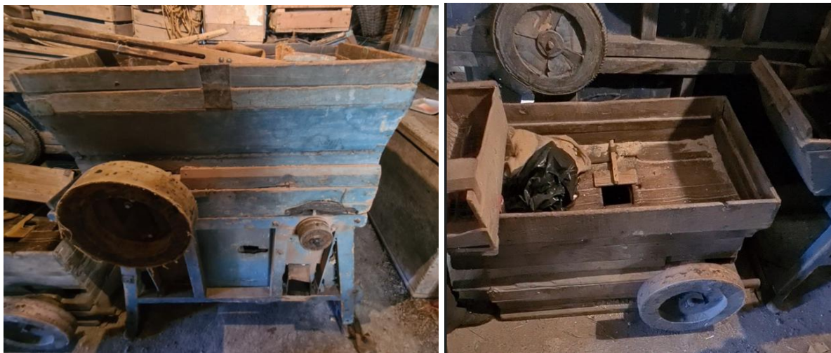
Fig. 4.1.7. G.F.'s chestnut beating machine on the left. The machine can be dismantled and converted into a maize threshing machine by replacing the upper part with the device shown in the photo on the right. Both machines were invented and constructed by Gino's father.
