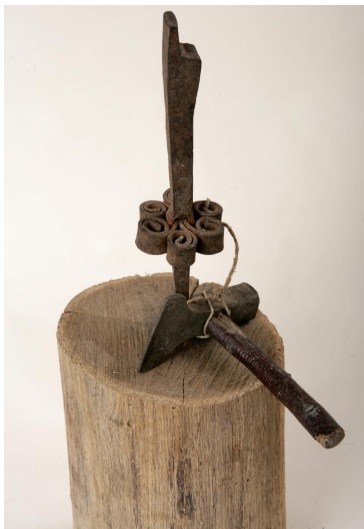
Fig. 4.1.5. a) Scythe ( scorriatte ) blades, for haymaking. b) A marcia – a small field anvil for peering scythes – and a small hammer. Source: Held at the Museo Contadino di Cassego. Photographs by Moreno Carbone.
