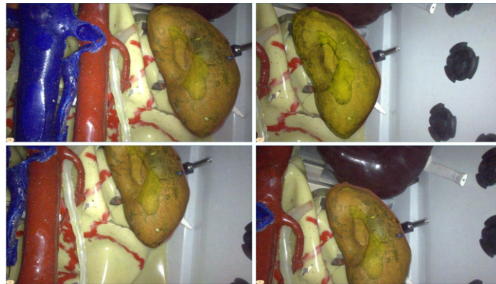
Figure 6.9 Sample images of the AR guidance visualization in four different positions of the teleoperated robotic endoscopic camera during the experiments. The kidney virtual 3D model remains overlaid with high accuracy on the image of the real organ independently of the position.
