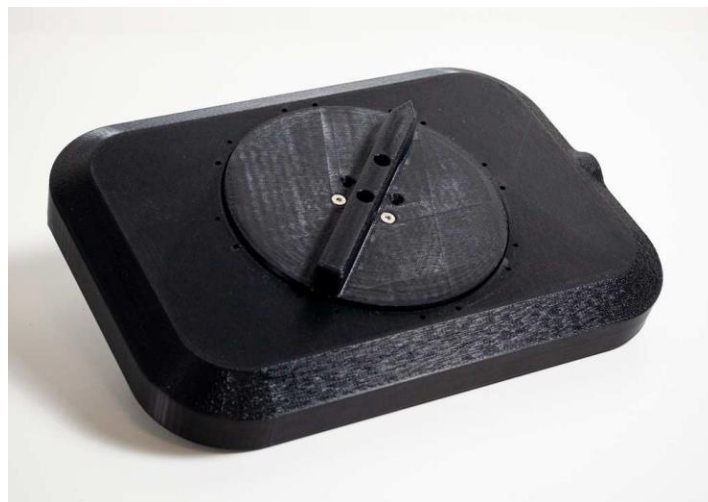
Figure 3.1. External view of the TaK device. The device consists of a 3D-printed base supporting a rotating circular board with an arrow-shaped tactile bar used to reproduce perceived orientations.
