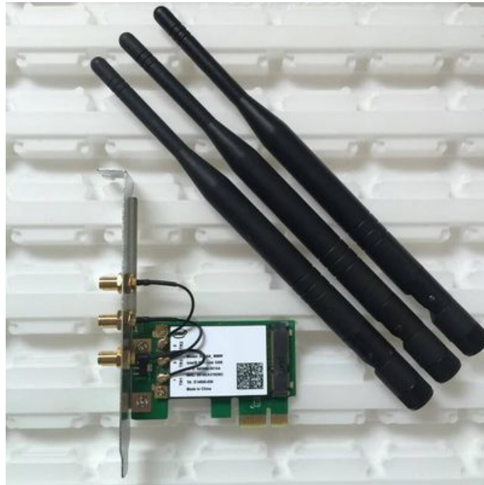
Figure 3.1: The Intel Wireless Wi-Fi Link 5300. This 802.11n device has three transmit/receive antennas, operates on both 2.4GHz and 5GHz frequency bands, and supports up to three spatial streams for a maximum bitrate of 450Mbps [5].
