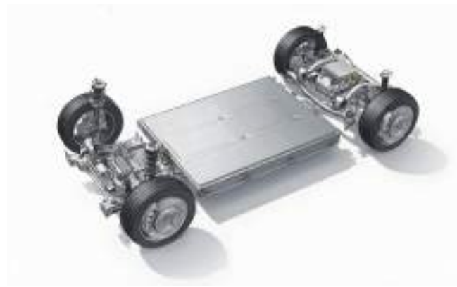
Fig. 10. MG4 Electric car platform (MG Motor Europe), original conceptual sketch (Musio-Sale, Peri)
