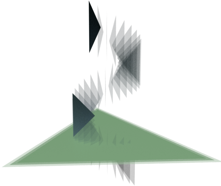
Figure 5.6: Test problem: CCD of a triangle moving rigidly along a screw trajectory, and another deforming triangle. The triangle on top rotates and moves along an axis until the two primitives come into contact.
