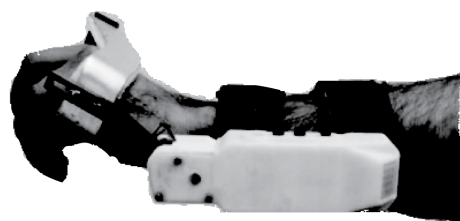
Figure 6. One DoF rigid wrist exoskeleton designed by [18]. Image adapted from [18].
