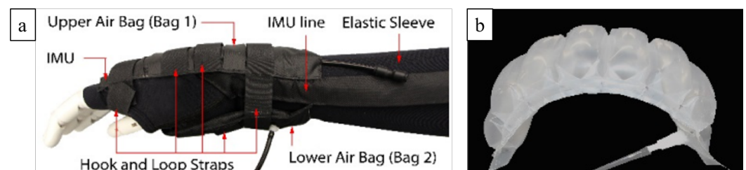
Figure 14. Soft wrist exoskeleton designed by [34] to alleviate CTS: (a) the whole device; (b) the airbag actuators.
