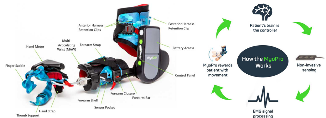
Figure 26. MyoPro device by Myomo, Inc., Boston, Massachusetts, US [32]. Images reproduced with permission from the company.
