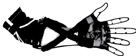
Figure 9. Soft robotic wrist orthosis [20]. Image adapted from [20].
