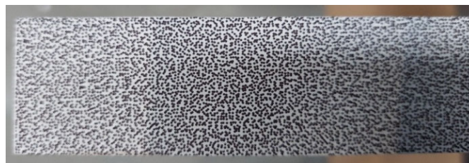
Figure 9. Speckle pattern points on the surface of a steel specimen.
