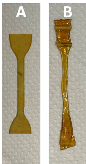
Figure appx. 3.8 PHTE-vitrimer sample before (A) after the DMA measurement (B).
