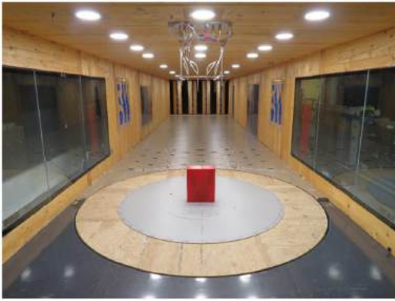
Fig. 2. Wind tunnel model and set-up tested by RWDI.
