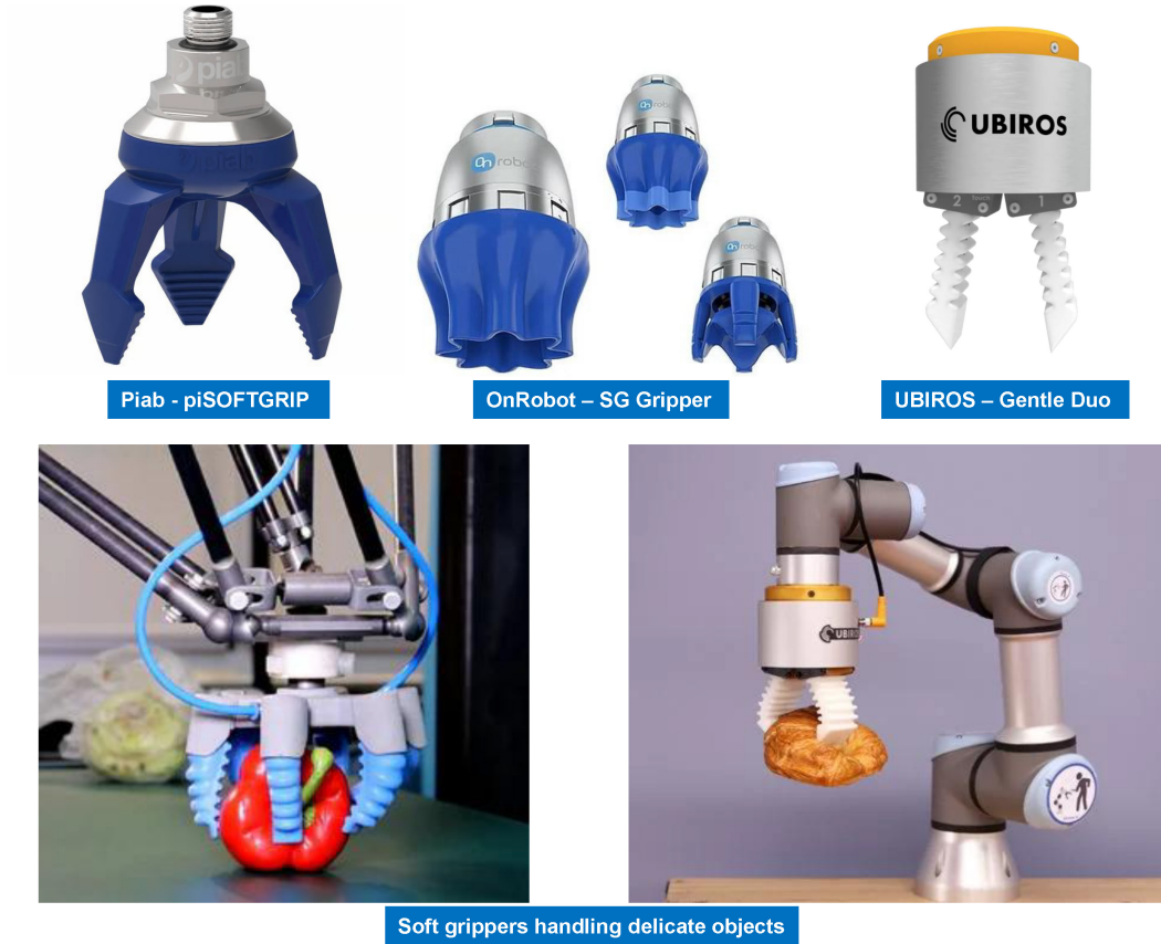
Figure 1.2: Examples of commercial soft robotic grippers and application of soft grippers in handling delicate objects
