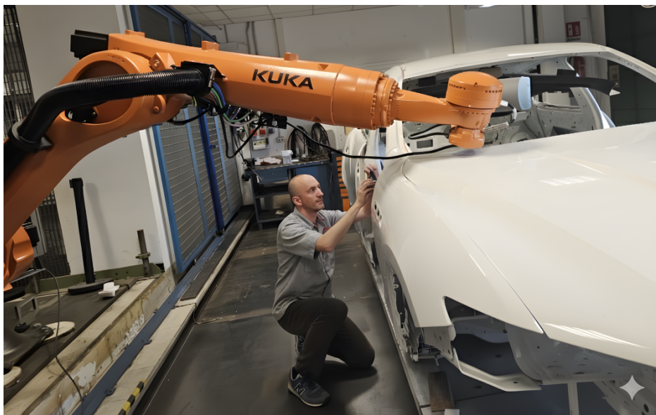
Figure 8.13: Proximity-based obstacle avoidance demonstration. A worker comes into the KUKA's workspace during programmed motion (Phase 3). The ToF sensors on the UR10e detect the intrusion, triggering graduated response: warning zone detection (200–500 mm) reduces velocity to 5% via Input 1, while danger zone detection (<200 mm) triggers complete stop via Input 2. The robot continues its programmed trajectory after obstacle removal (person leaves the warning zone) without requiring manual repositioning or program restart.
