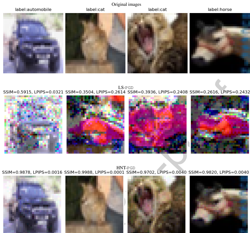
Figure 6: Visual comparison of adversarial examples generated by LS-PGD and HNT-PGD on CIFAR-10. The top row shows the original clean images. The middle row displays the adversarial examples from LS-PGD, and the bottom row shows those from HNT-PGD. The SSIM and LPIPS perceptual metrics are reported for each generated image.
