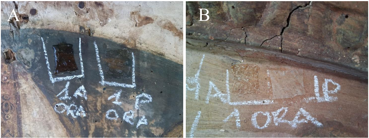
Figure 46- Repainting (A) and aged varnish (B) areas with application of Agarose/PEO (left) and PVA (right) mats.
