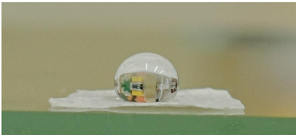
Figure 66 - Macroscopical hydrophobic behaviour of PCL electrospun mat
