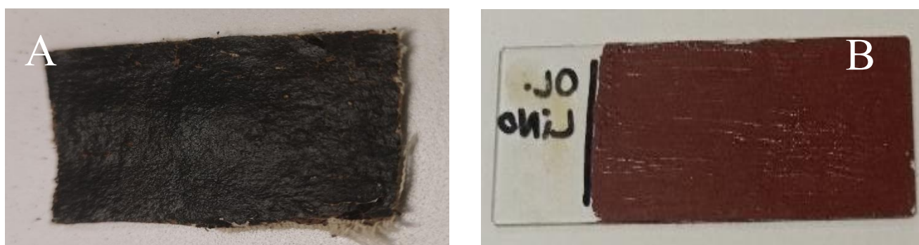
Figure 34- Reference surfaces for deswelling test: (A) pieces of tempera on canvas and (B) painted glass composed of linseed oil and iron oxide-based pigment.
