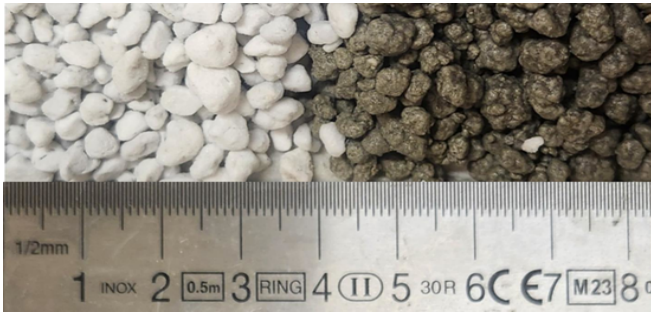
Fig. 1. Perlite aggregates (left caption) and PCM-enhanced aggregates (right caption).
