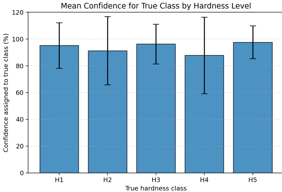
Figure 3.13: Mean confidence assigned to the true hardness class for each hardness level (H1–H5), with error bars representing the standard deviation across windows.
