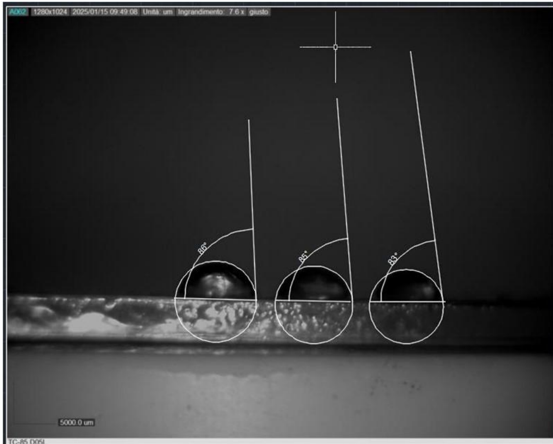
Figure 9-2 Direct printing sample, with 3 drops of physiological saline solution and respective contact angles
