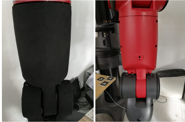
Figure 4.18 Figure on the left represents Baxter's arm with old electronic skin; on the right the same arm without electronic skin. The red part is the aim of the prototype.
