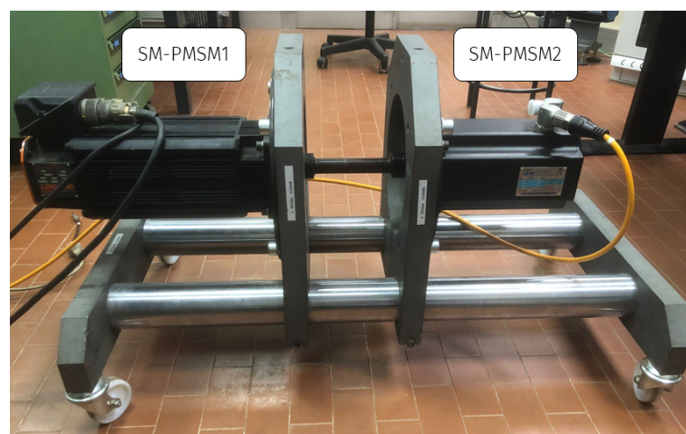
Figure 5.6: Experimental setup, SM-PMSM motors
