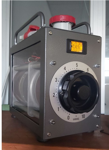
Figure 5.7: Experimental setup, variac
