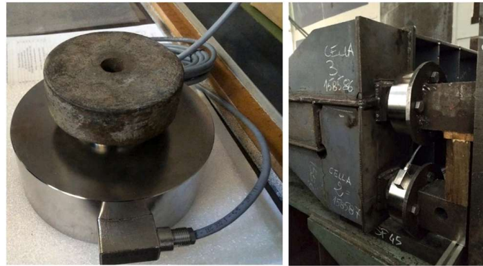
Fig. 13. Load cell heads with ball joint coupling (a) and position of the load cells (b).
