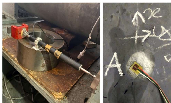
Fig. 14. Potentiometric displacement sensor (a) and strain gauge rosette with 3 acquisition channels (0°, 45°, 90°) (b).
