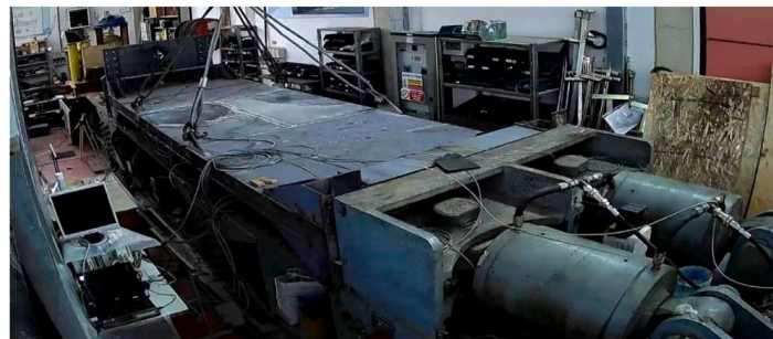
Fig. 12. Panel setup, view from the moving edge which translates axially thanks to the two actuators.
