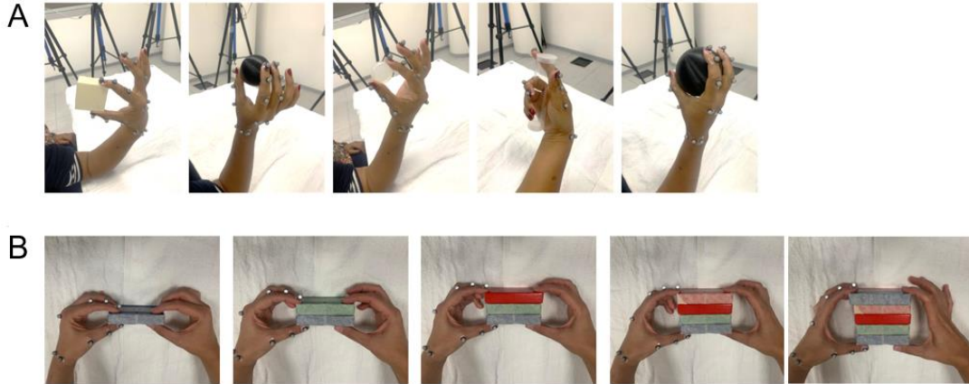
Figure 5.3 – Objects grasp for Task 2 and Task 3. (A) Hand grasping various objects (cube, plug, cylinder, two spheres) during Task 2, with reflective markers on the hand. Colors are arbitrary; the cylinder is transparent for HL2 marker visibility. (B) Top view of lateral pinching of a rectangular object with varying thickness during Task 3 (one hand tracked with VM while the markerless one tracked via HL2). Thickness increases by 2 cm per added segment; object colors are arbitrary.
